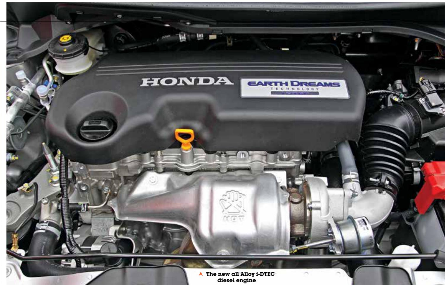
▲ The new all Alloy i-DTEC diesel engine
